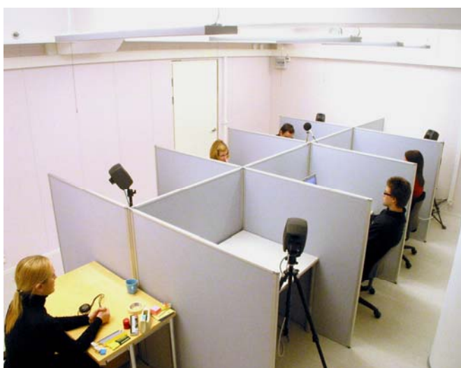
Figure 1: The office laboratory (30 m 2 ) contains 8 workstations. Four subjects were tested simultaneously and they sat in the middle. Speech was produced from four other workstations in random sequences. Masking sound was produced from four loudspeakers hidden above the suspended ceiling.
