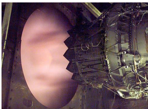
Figure 4: F135-PW-100 engine test illustrating noise-reducing chevron nozzle implementation in a high-performance jet engine (courtesy wikipedia)
